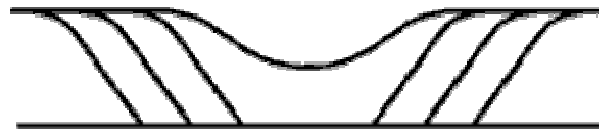
Figure 4 - With increased cutting laser power the pits become wider while maintaining a constant edge slope
