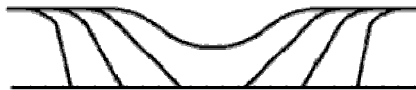
Figure 5 - With increased developing time the pits become wider with steeper edge slope
